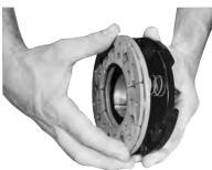
**ACAUTION** Straight springs must fit into grooves in armature hub.
